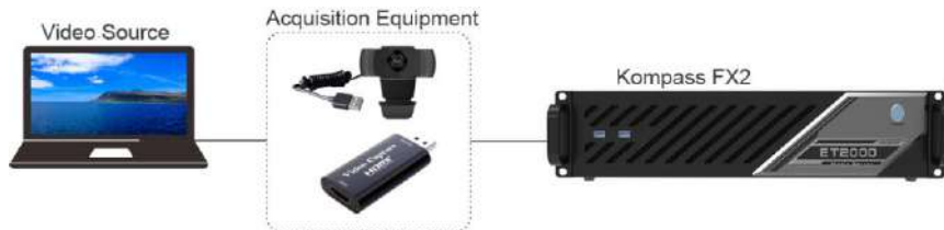
Figure 5-13 Data acquisition connection
